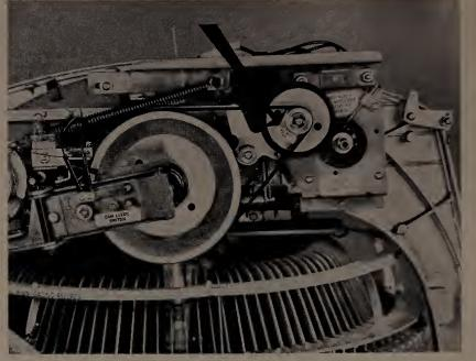
Top-rear closeup—bearing is positioned in center (hidden) of small drive wheel immediately top and right of sign reading DO NOT OIL (see black arrow).
