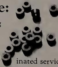
Instead of moving parts, TORMAT uses scores of tiny, doughnut-shaped memory cores called toroids. These solid "doughnuts" remember selections electronically and pass them on at the proper time.
