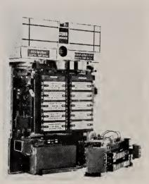
Photograph shows a Wurlitzer wall-Photograph shows a Wurlitzer wall-box open for servicing. This wallbox is still operative, even though a serv-iceman may be working on it. If a coin has been inserted and a selection made, the box will function though the front assembly has been removed. This feature is built in all current Wurlitzer Wallboxes, with or without
