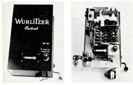
Wurlitzer 'Cashrak' (left), was introduced to distributors this month during summer meetings. Right, exposed coin counter has two prongs-one to power source and one to playrak. Two screws hold the unit in place.
