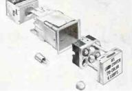
The IEE 'Lumi-Switch' Six-Lamp Push-Button Switch Unit. released recently by the Industrial Electronic Engineers, Inc., offers three colors (two lamps per color), several other color-lamp combinations, and a num-ber of horizontal and vertical split-face options. The unit is .965 in. high, 1.205 in. wide and features a push button viewing screen that is .75 in. high and .28 in. wide. The legend may either be engraved or put on film be-
