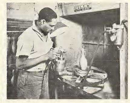
Pins are produced by Chicago-Allis Corp. Pins are spray coated with flexible Chemglaze coating (above).
