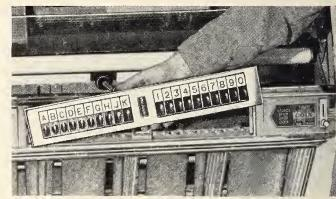
Key panel is simply removed by releasing two sliding lock fasteners.
