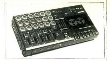
he Porta 05 mixer is a 4-in/2-out design that offers plenty of versatility for both recording and playback. All four inputs accept line-level input from electronic instruments as well as standard signal processing devices. Input channels 1 and 2 also accept microphones for recording vocals or acoustic instruments or direct inputs from electronic instruments such as guitars. Trim controls are provided to set the optimum input level.
