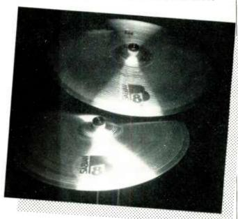
Introduced at the summer NAMM, the new Sabian B8 and B8 Plus are both European style cymbals. This means they are spun-formed to the cymbal shape from a B-8 bronze alloy disc (92% copper, 8% tin). Sabian's cymbal makers have so dramatically improved this forming process that the B8 and B8 Plus offer what the manufacturer refers to as "exceptional sound quality and durability for a remarkably low price."
