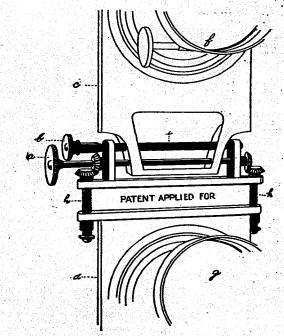
New device for registering the position of the upper lantern of a dissolving stereopticon to obtain perfect registration on the curtai
