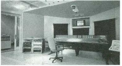
The control room at the Dairy in London, featuring a DDA AMR 24 36/24/24/2 console with Optifile Tetra automation, ATC SCM 200 monitors, and outboard gear from Tubetech, Focusrite, Valley People, Lexicon, and others.
