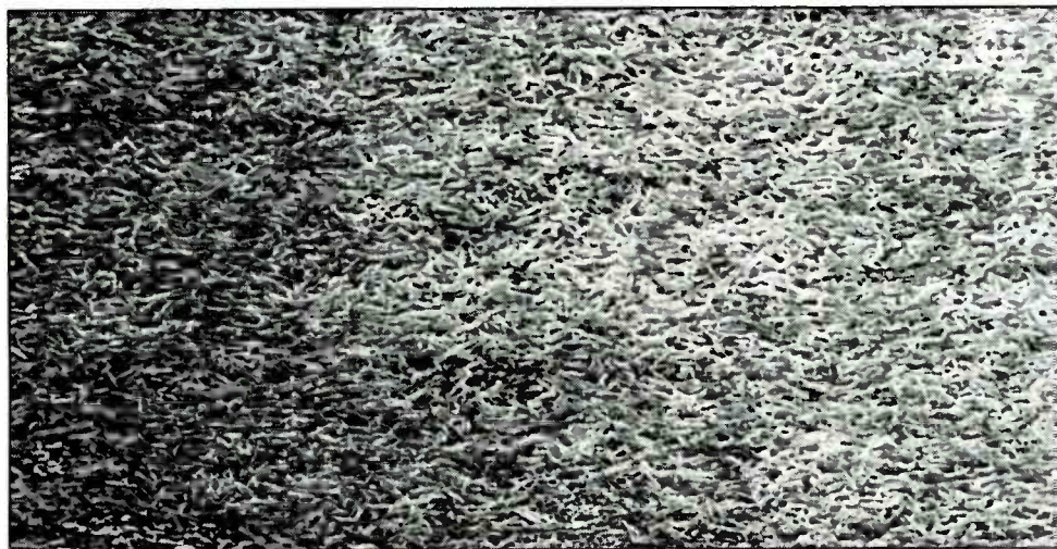
Magnified magnetic particles from the surface of TDK's new Pro Cobalt (APG) tape
