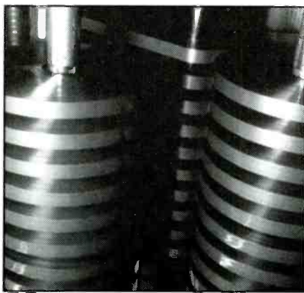
Rewinder turning slit tape into pancakes
