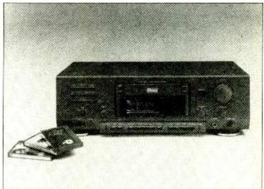
A prototype digital compact cassette (DCC) unit from Philips
