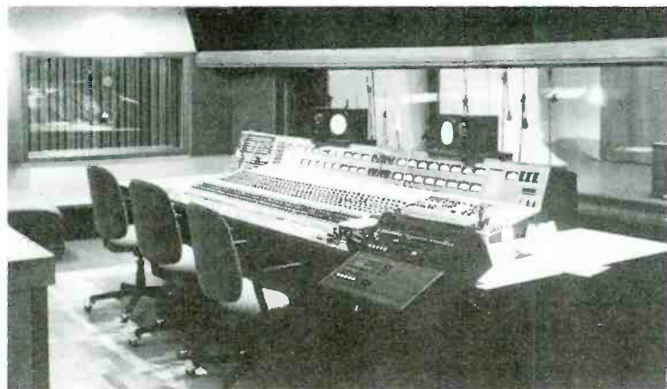
The control room for Criteria's Studio A, above, features the Neve 8078 console and three-tier ceiling design by George Augsberger.
