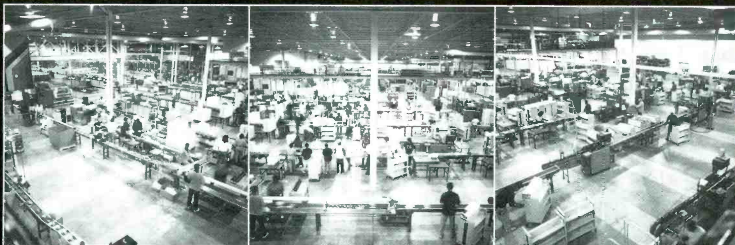
Technicolor Videocassette packaging areas are designed for speed and accuracy, and include labeling, stickering, shrink-wrapping, security, and bar-coding.
