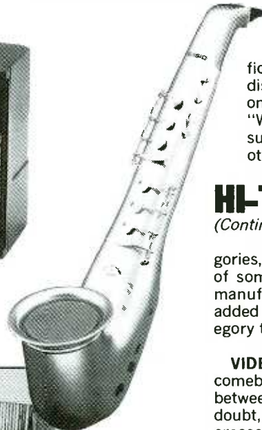
Casio's DH-100 digital horn with six built-in sounds, recorder fingerings and breath activation.
