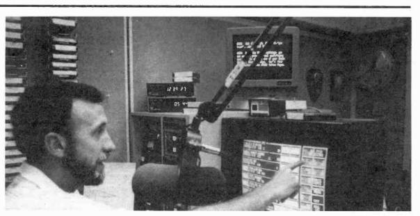
The new touch-screen system in use at WEEI Boston allows computerized broadcast control, enabling stations to keep records of aired commercials in an easier and more accurate manner as well as performing other functions.
