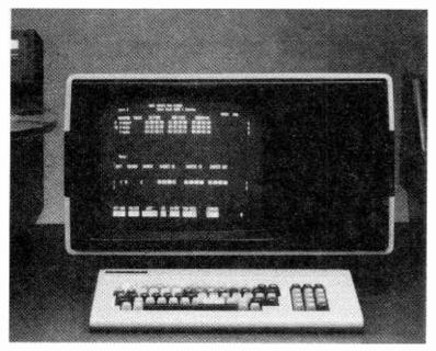
CMX Corp.'s CASS 1 Computer-Aided Sound Sweetener claims to be the first intergrated time code-based audio editing/console automation system. It can simultaneously control up to six ATRs and 15 additional sources to allow mixing of an entire sound track. Cost is \$40,000 and up.
