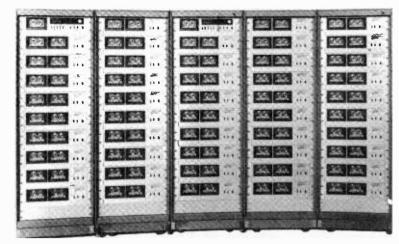
**Reel-ly Making Time.** Kenneth A. Bacon Associates (KABA) will display its 50deck, four-track real time cassette duplication system, claimed to differ in several ways from the practice of using consumer decks for real time duping. KABA says the system shown will produce 3,000 C-45s per shift when used in the three and three-guarter i.p.s. mode. System prices start at \$2,270.
