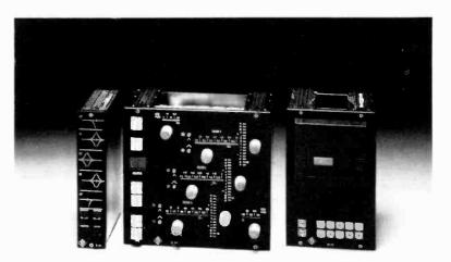
**Microchip EQ.** Gotham Audio Corp. will show Neumann's new AME automated equalizer system with 64-channel capability. The AME features data cassette storage, archiving of console settings, A/B comparisons for every channel and master/slave operation for the formation of stereo channels or groups. See it at Booth 221.
