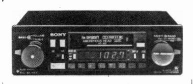
Sony Car Stereo's XR-100 model uses the diversity reception system to eliminate multipath distortion that occurs when direct and reflected FM signals are picked up at a single antenna. By placing two antennas in separate locations, the XR-100's microprocessor constantly uses the strongest signal. The unit also features an auto reverse cassette deck with an amorphous tape head. It retails for \$649.95.
