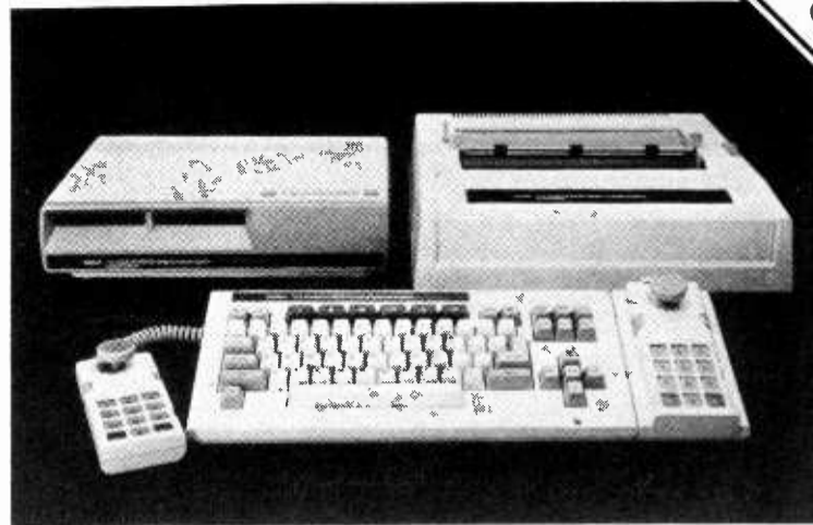
FAMILY MAN —Coleco announced the birth of Adam at CES. The "family computer system" includes an 80K memory console, printer, a 75-character keyboard and two keypad/joysticks for game playing.
