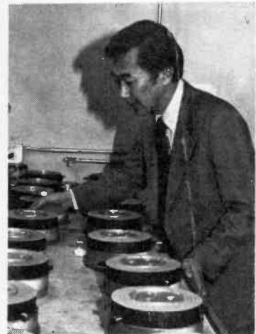
Special Spiders: Voice coil wires are wrapped around "spider" holders before being connected to the speaker cones at the Cetec Gauss factory.
