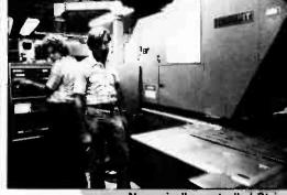
Numerically controlled Strippit (above) punches sheet metal at a rate of over 200 holes per minute.
