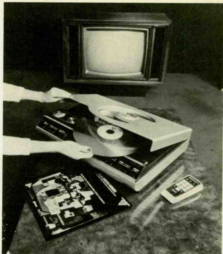
Videodisk Debut: Production model of Magnavox-built optical videodisk player for Philips/MCA system gets a tryout.
