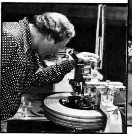
Phil Cross, mastering engineer at Filmways / Heider follows a direct-to-disk lathe cutting.
