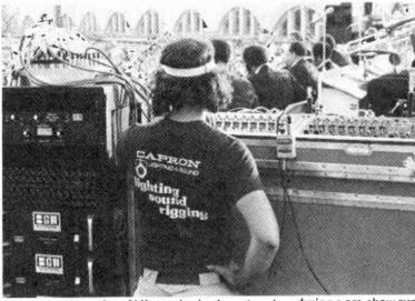
Capron monitor mixer Al Kennedy checks out system during a pre-show runthrough. Visible are the UniSync Trouper I mixer, in its road case, and some of the BGW power amps used in monitor and house setups.
