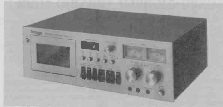
▲ TECHNICS RS-671US front-loading stereo cassette deck has 2 motors, 2 heads, bias/EQ controls, memory rewind, solenoid controls.
