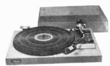
▲ TECHNICS SL-23 is frequency generator, servo-controlled belt-drive semi-automatic turntable with strobe, electronic speed switch.
