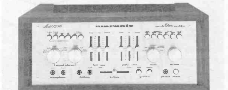
▲ MARANTZ 1250 stereo console amp delivers 125 watts RMS per channel, has separate record mode selectors/monitors for two tape sources.
