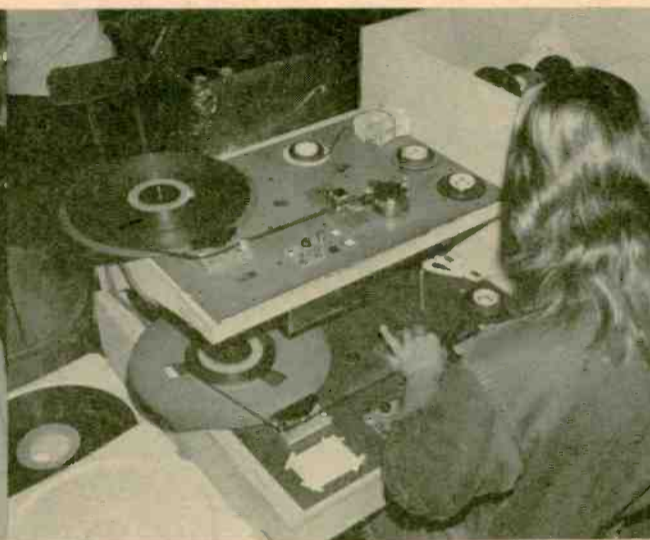
JANE SORENSON is operating an LTD CW25 loader, loading platforms with pre-recorded tape from bulk hubs. Note the dual take-up hubs for continuous operation.
