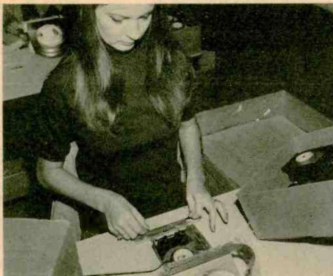
Delicate operation of splicing an 3-track cartridge is handled here by LUANN NEVE. The cartridge at this point has just left the winding station.
