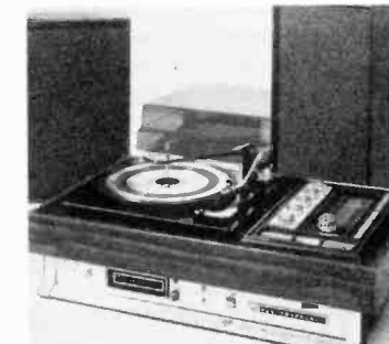
MORSE ELECTRO PRODUCTS Quadri-Stereo W92612K includes 8-track recorder/player, AM/FM stereo radio, BSR changer, two microphones, dust cover, and two 6 in. fullrange speakers. The Electro-phonics matrix system retails at $209.95.
