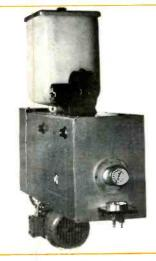
Fabelmix • Adjustable speed and output • Monobloc unit with any press • Horizontal extrusion • Economical and quick steam heating • Use of material under several shapes (dry blend, pellet, or regrinds) • 45 gr in 12 seconds • One hand operation
