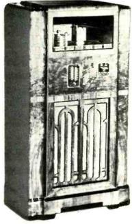
ROCK-OLA ENTERED the coin-operated phonograph field in 1935 with the introduction of this 12-play Multi-Selector unit. Records were easily accessible through the front door and record damage was minimized by reducing the weight of the pick-up to only two ounces.
