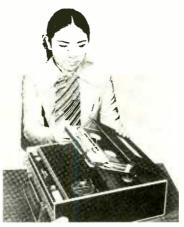
PANASONIC introduced a new two-reel magazine loading color video tape recording system two-reel magazine loading color video tape recording system based on the cassette principle Nov. 10 at the convention of the National Association of Education Broadcasters. The unit is capable of recording and playing back both color and black and white images on ½-inch video tape magazines. Panasonic hopes to market this by 1972.
