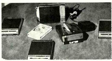
PANASONIC'S 8-track cassette adapter is seen here surrounded by other prototype models. At rear, a transceiver pack for citizens band communications. The three units at the edge of photo are among a group of seven tuner packs that include short wave, long wave, marine band, AM, FM/FM, AM/FM and FM tuners.
