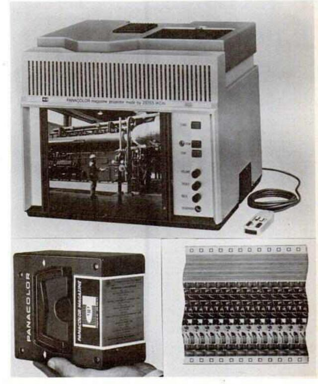
PANACOLOR FILM CARTRIDGE SYSTEM utilizes a 12-track capstanoperated mechanism. The unit functions with a magazine-type cartridge which automatically feeds the film into a take-up reel within the projector. Film format utilizes 12 rows of picture images and 12 rows of optical sound tracks. Width of film is 70mm.
