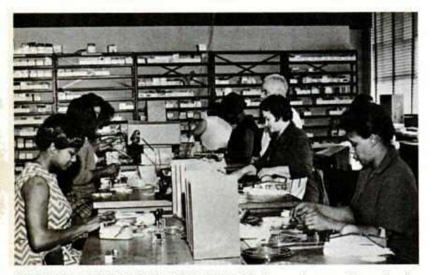
WINDING TAPE INTO CARTRIDGES from the pancake reels du-
