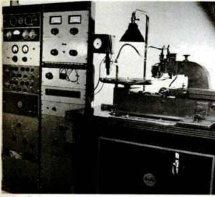
SCULLY CUTTING LATHE, from which most of Bell Sound's master lacquers are prepared.
