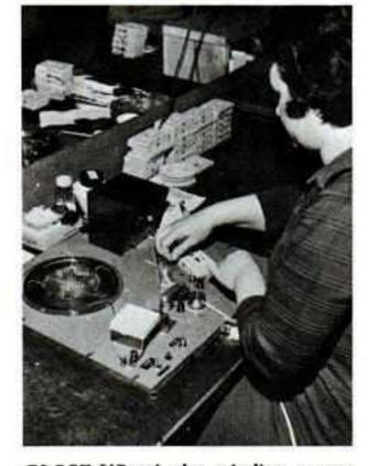
CLOSE-UP of the winding procedure done on A&B's automatic unit,
