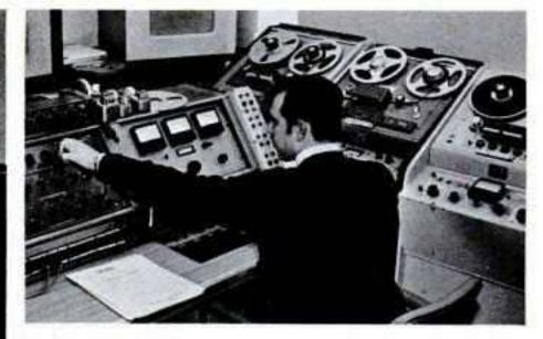
REMIXING. Engineer reduces the multi-track tape to 2-track stereo and monaural.
