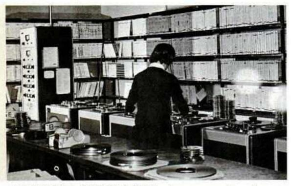
A&B's SECOND DUPLICATION line features a reel-to-reel master controlling 10 slaves for duplication of 4-, 8-track and cassette production. All slaves are equipped with interchangeable plug-in head assemblies, permitting the same equipment to be used for all configurations.
