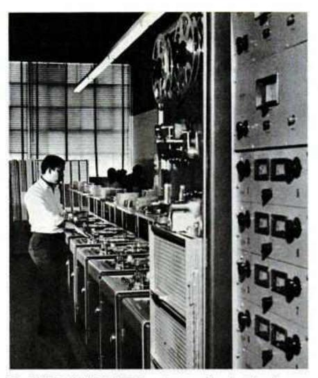
MASTER PLAYBACK rolls tape for duplication on 10 slave units. A&B's capacity for 8-track cartridge is 18,000 per shift; 9,000 for 4-track and cassette. The master unit utilizes a continuous loop master regardless of configuration, thus providing for minimal production time loss.
