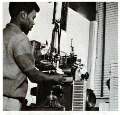
AUTOMATIC LABELER, neatly and precisely, gums cartridge slick onto cartridge. One of four machines, this automatic device's capacity is 6,000 labels per shift.
