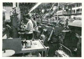
A record presser "dinks" a disc. The fist-full of compound is placed in a machine, flattened, grooved and center-holed in one operation, and then trimmed in another. Then the label goes on. It's all done in seconds.
