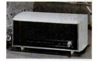
OPERATING ON BATTERIES or AC, this Arvin radio (Model 28R17) retails for a suggested price of \$14.95. It is a solid-state model with seven transistors and encased in off-white plastic.
