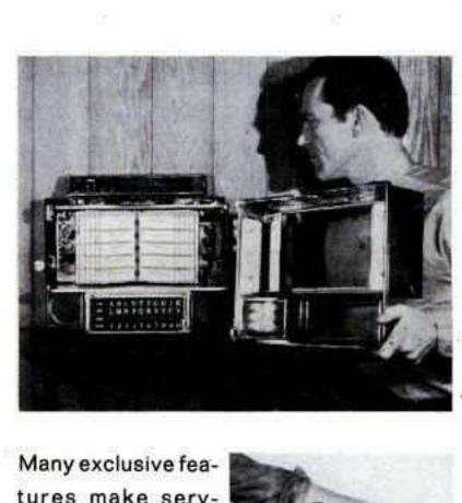
Many exclusive features make service a breeze. When used on counter, the Wall-Ette can be serviced from back without disturbing customers.
