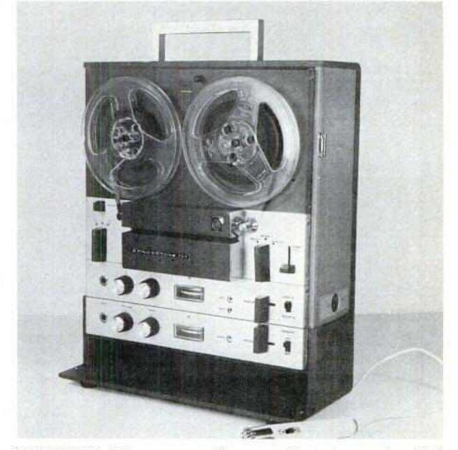
CONCERTONE 727, a new cordless portable tape recorder which operates on standard AC as well as "D" cell dry batteries is an example of the type of increasingly popular tape equipment which will be displayed extensively at Chicago's Music Show in July.
