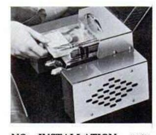
NO INSTALLATION, autosonic, four-track stereo tape deck by Martel Electronics. Fits hump on floor of any car; plugs into cigaret lighter. Can be attached permanently if desired. AC converter available, plays in car, boat, on beach or patio. No price.
