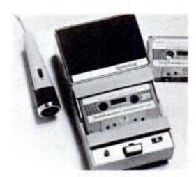
WOLLENSAK manual cordless cartridge tape recorder by the 3M Co. Solid-state capstan driven transport, single switch controls record, playback and fast search functions, dual purpose battery condition/recording level meter. Remote control playback and recording in microphone switch, operates on five C batteries at 17/8 i.p.s. Price \$99.95, including case, microphone, batteries and three tape cartridges.
