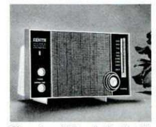
Champion AM radio by Zenith. Filter magnet antenna screens out static, tuned RF stage with 3-gang tuning condenser. Illuminated slide-rule dial, tone control. Polystyrene cabinet with grained wood panels, finished back, recessed handle. Price \$43.95.
