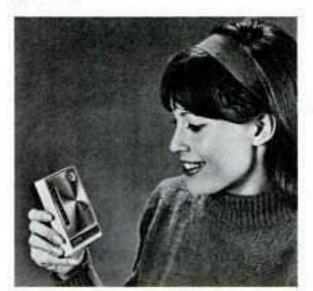
Shirt-pocket 8-transistor radio. Slide-rule dial, wavemagnet antenna. "Squeeze lite" feature; press sides of cabinet to light up dial, release to put out. Cycolac cabinet. Price \$18.95 includes case, earphones and batteries.
