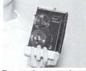
Two pound tape recorder records one hour in each direction by Concord Electronics. Solid state and flux-field head achieve sound at 1-7/8 IPS, tapes interchangeable with larger recorders. Uses 1/4 mil tape with optional voice-operated microphone. No price.
