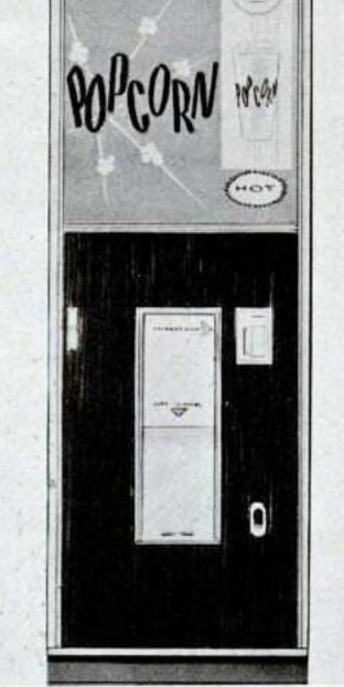
POPCORN VENDER manufactured by Gold Medal Products Co. of Cincinnati. Model 300, modular for bank vending. Front load service with 175 capacity at 18 ounces per serving. Uses Merkle-Korff Pos-Adjust cup drop. Adjustable National Rejector to sell at dime or 15 cents. Coin changer optional. Illuminated display built into a wood grain finished front panel.
