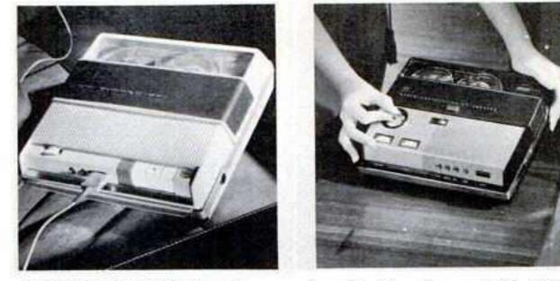
WEIGHING LESS than five pounds each, these two portable RCA tape recorders are battery operated. Both are reel-to-reel recorders with recording/playback speeds of 3-3/4 and 1-7/9 ips. The model on the left uses four batteries and is priced at \$49.95. The six-battery model on the right has a price of \$65.00.
