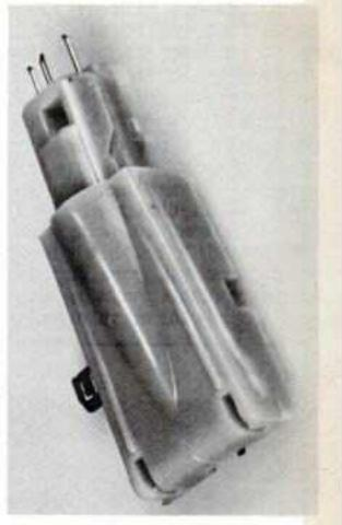
JENSEN INDUSTRIES' new X3D phonograph cartridge provides a central sound channel (in addition to stereo right and left) which blends the two stereo channels. Cartridge is designed to service a third center speaker.
