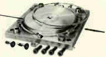
« FABELMO » dies, with interchangeable forged chrome nickel steel heating plates
