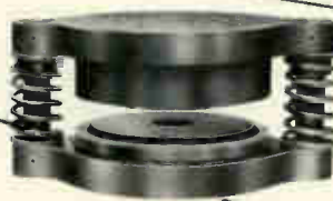
« FABELFO » stamper forming tool for each size and separate forming tool for conical centers
