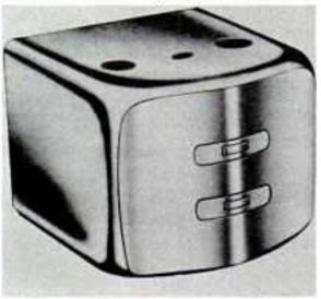
The Nortronics Company, Minneapolis, has introduced a new eight-track stereo tape head for 1/4-inch tape, designed to offer twice as much playing time as the standard four-track stereo tape system at the same tape speed. Called the Model B2L, it has a 100-micro-inch gap and the head is mechanically indexed to four discrete positions to provide four stereo or eight mono channels. It will be available in either solid or laminated core versions.
