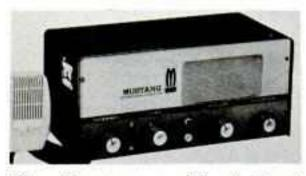
The Mustang, a citizen's band transceiver, has been introduced by Metrotek Electronics, a subsidiary of Regency Electronics. The unit has six crystal-controled transmit channels and may be tuned to receive all 23 channels. It transmits on any six of the 23 available CB channels. Plug-in crystals, mounted on the chassis, can be changed to provide any desired frequency. Power output is 3.0 watts, minimum. A high impedance ce-
