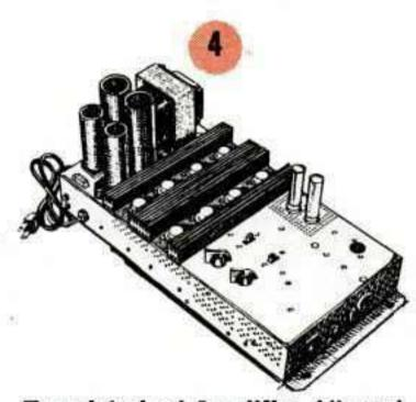
Transistorized Amplifier All new! Provides lifelong service for phonograph. Saves money on tube replacements. Elimination of excessive heat saves wear on other components. Noise suppressor automatically eliminates surface noise. Circuit protector bulbs prevent damage to transistor if speaker leads should be shorted:
