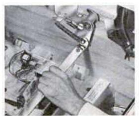
PLAYBOARD AUTO-CLAMP—No more screws to hold the playboard! Just pull the lever and lift the board! Gives immediate access to interior mechanism. Truly a service man's dream.
