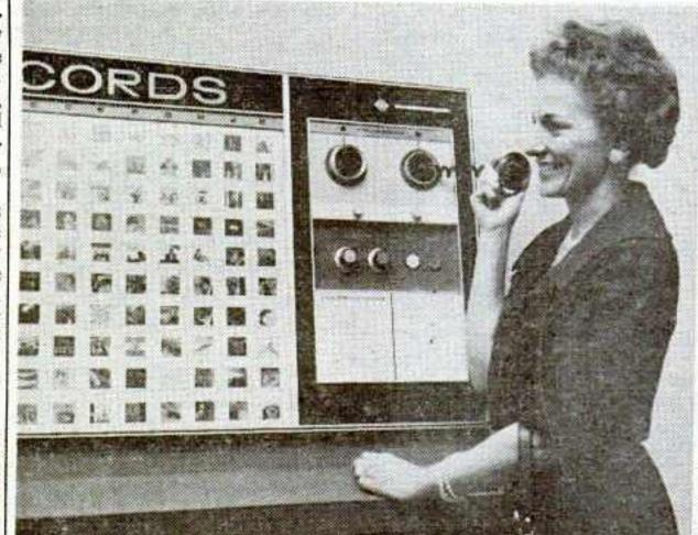
STORE CUSTOMER IS PICTURED about to listen to her selection on the Recotron, disk audition unit. Pull-out earphones are available for both stereo channels, while knob controls (middle left) allow selection by number and letter combination as in juke boxes. Reject button at middle right allows selection change at any time, rather than at conclusion of selection only.
