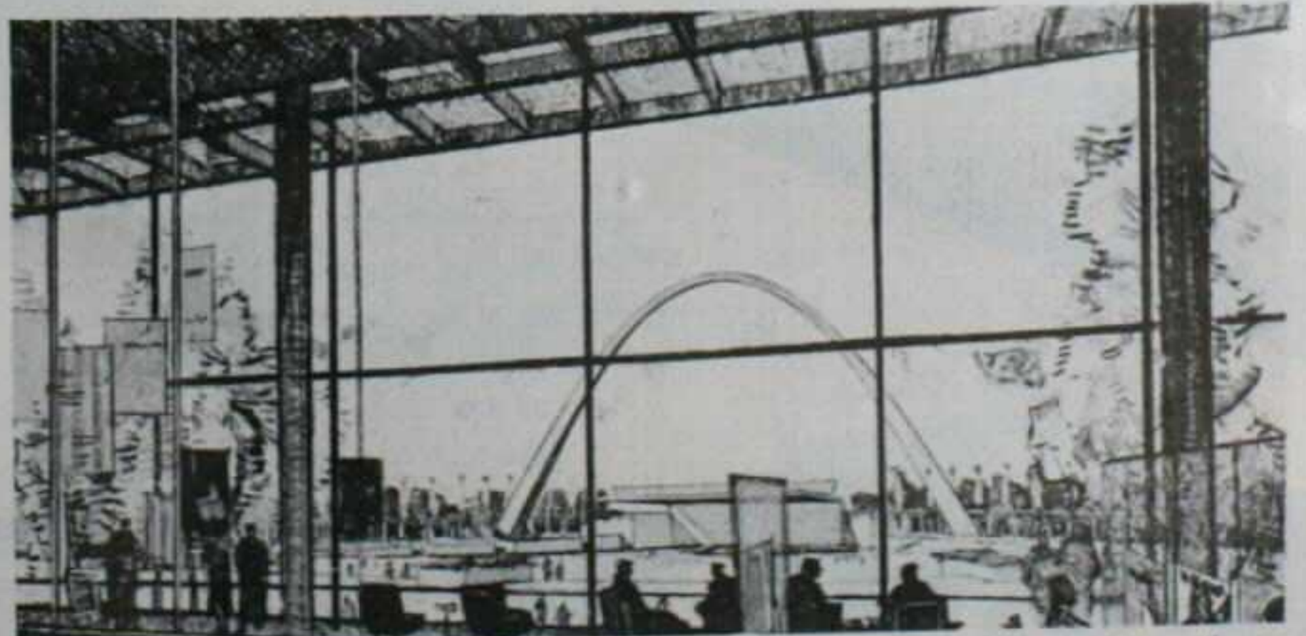
A recent artist's sketch of the State Exhibits building is shown above. The structure rides on ground-free columns, forming both the backdrop and forecourt for the theater. Altho the building is raised one level from the ground, it is typical of the construction of the exhibit buildings—light, open, simple, informal and unpretentious.
