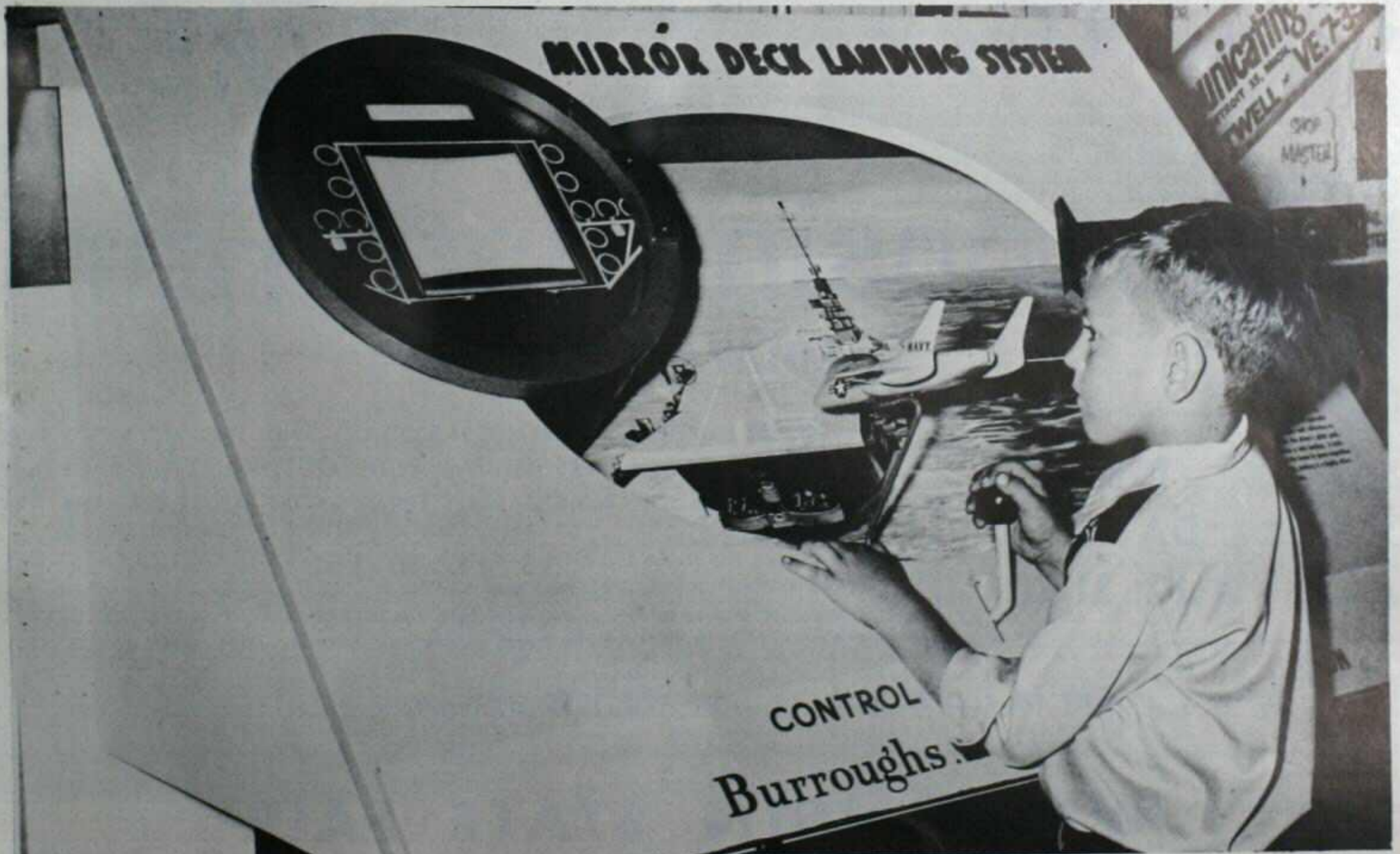
A Burroughs Mirror Deck Landing System for airplane carriers was one of the most popular features of the made-in-Michigan electronics equipment show at the '58 Michigan State Fair. Fairgoers, such as the youngster above, were invited to manipulate a model plane. A light spot on the mirror at one corner indicates the plane's position in relationship to the landing strip on the carrier.
