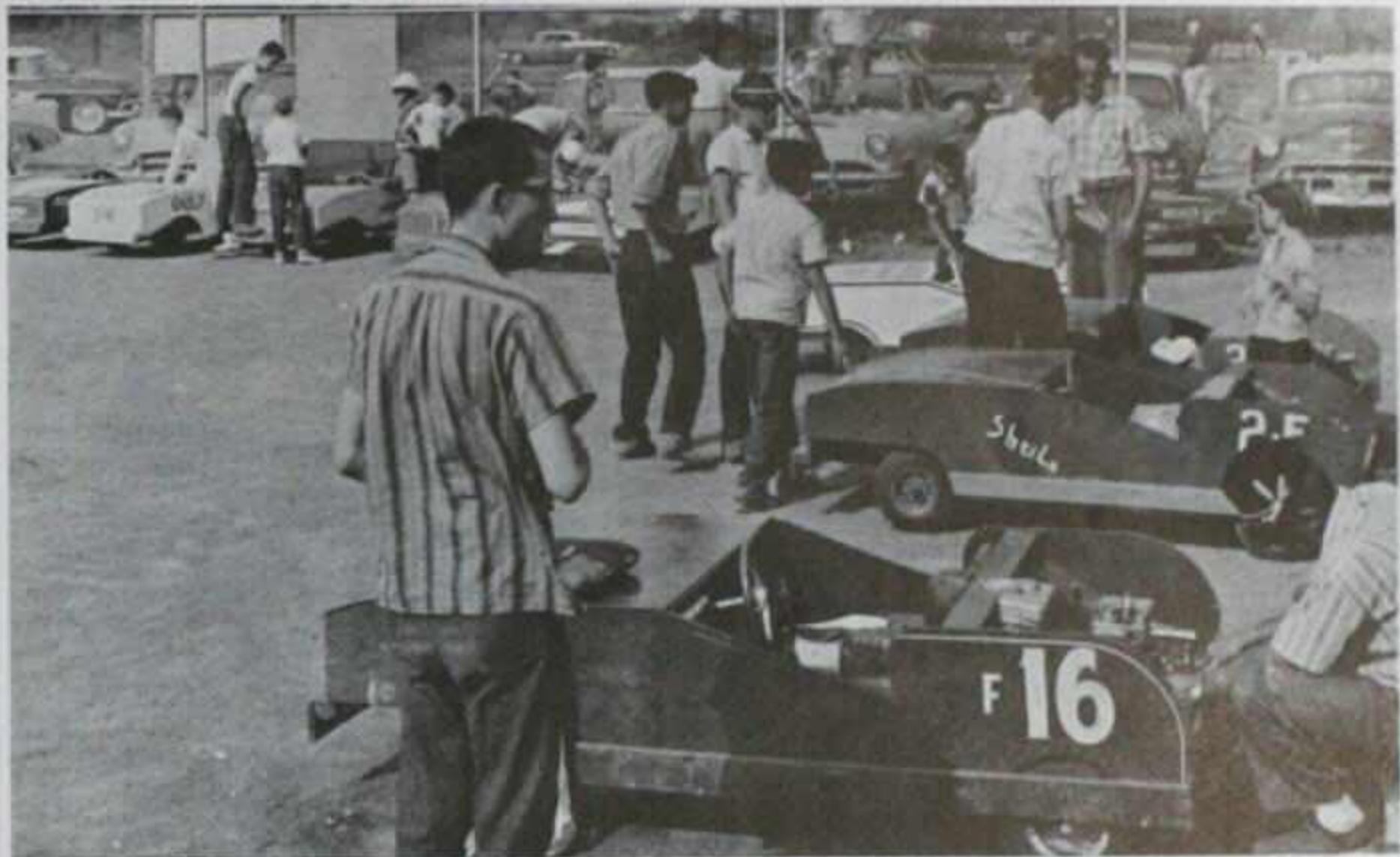
Scene in the pits has big-time racing flavor and shows some of the microd construction details. Motors are kicked over by cord, like outboard motors. Youngsters gain mechanical knowledge ahead of their years from this craze.
